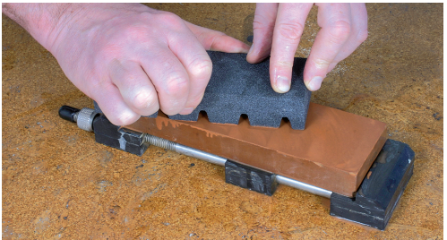
Fig. 13: Truing a sharpening stone with a ceramic truing block
