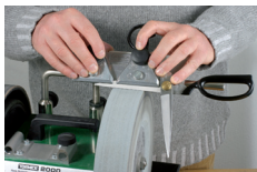
Fig. 26: Sharpening with a Tormek® sharpening machine
