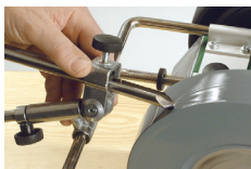
Fig. 23: Sharpening a bowl gouge using the gouge jig of a Tormek® sharpening machine
