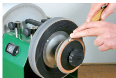
Fig. 22: Finishing with the Tormek® profiled leather honing wheel
