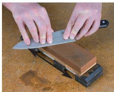
Fig. 2: Sharpening the back of the blade
