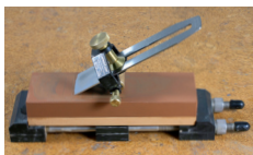
Fig. 19: Sharpening with a honing guide
