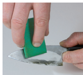
Fig. 11: Cleaning with the "rust eraser"
