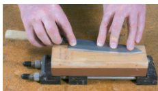
Fig. 5: Grinding a single-bevel blade
