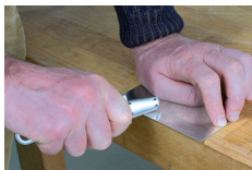
Fig. 24: Turning the burr with a Carbur burnishing tool (No. 703533)
