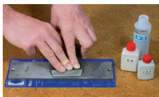
Fig. 14: Straightening the blade with a steel lapping plate
