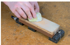
Fig. 18: Using a Nagura stone to create a polishing paste
