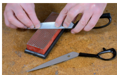
Fig. 25: Sharpening with a diamond block (No. 705367)
