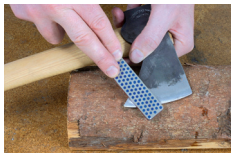
Fig. 27: Sharpening an axe with a multipurpose diamond sharpener
