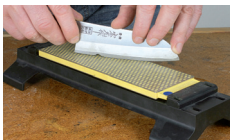
Fig. 7: Using a diamond whetstone
