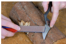
Fig. 28: Sharpening a pruning-shear blade with a diamond stone
