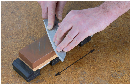
Fig. 1: Sharpening the front of the blade
