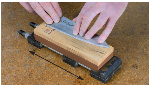
Fig. 4: Honing the blade lengthwise
